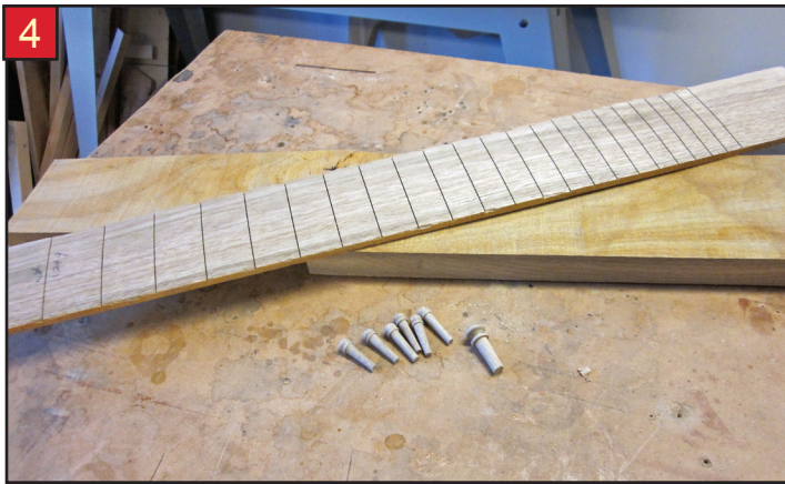
Persimmon fingerboard, bridgepins and end pin are all handmade
