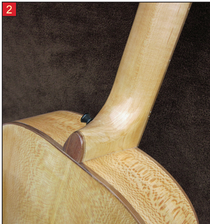
The Walnut heelcap and binding of the guitar show up well against the light wavy patterns of the sycamore
